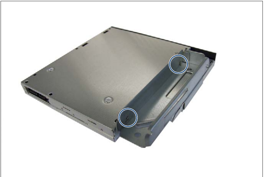
Figure 75: Installing the ODD
